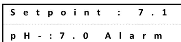
Figure 8 – Main Menu with an Active Alarm
