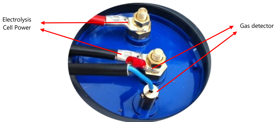
Fig 5 – Electrolysis Cell Connection Terminals
