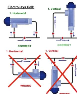
Fig 3- Electrolysis Cell
