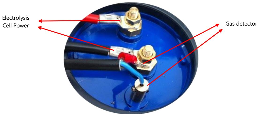
**Fig 5 – Electrolysis Cell Connection Terminals**
