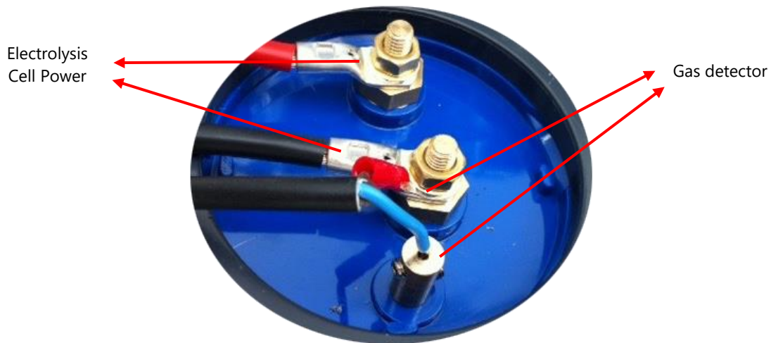
Fig 5 – Electrolysis Cell Connection Terminals
